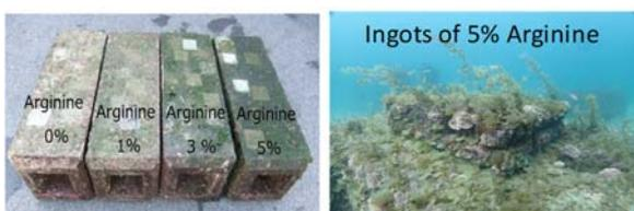
Fig.13 Concrete mixed with amino acids has a large distribution of micro algae
